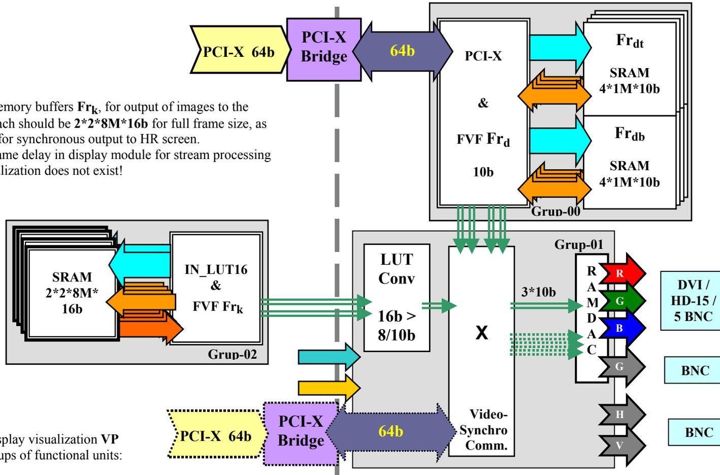
The module for display visualization VP consists of two groups of functional units:
