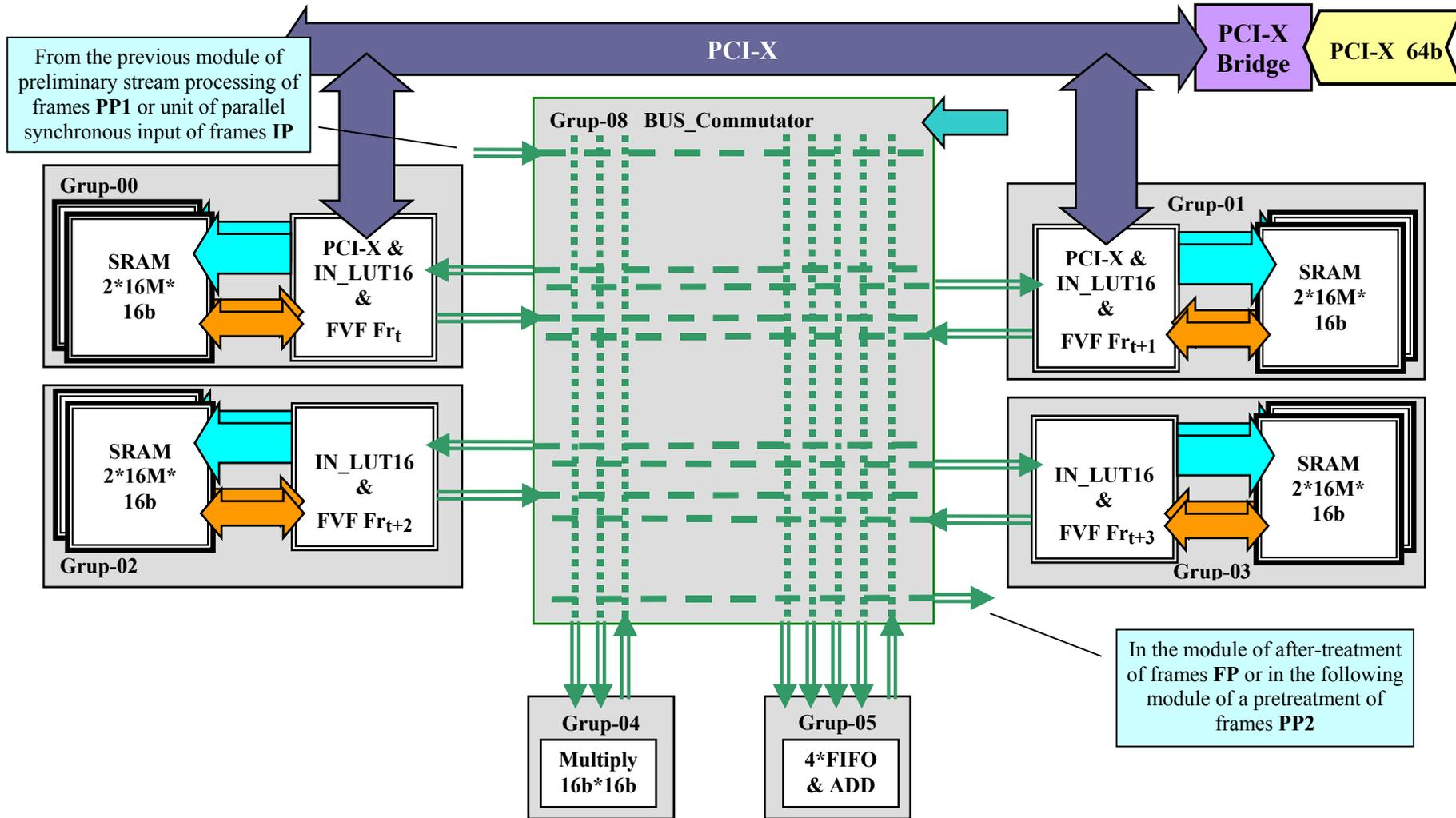
The input frame buffer FE  $FVF Fr_t$  and up to output frame buffer FE  $FVF Fr_t$  is double memory buffers, each of the full frame format.
