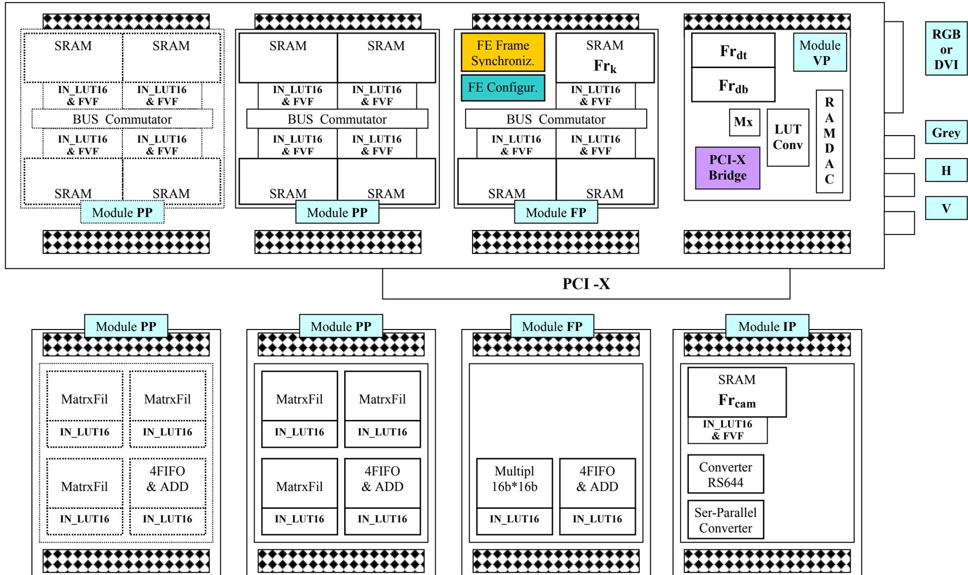
All modules, except configuration functional elements and frame synchronization for display visualization fit into “mezzanine” architecture. Such construction implies subdivision of elements placement at mezzanine (processing elements) and on mainboard (communication/link elements with frame memory arrays and handling elements). Mezzanine also features module of synchronous input from digital camera.
