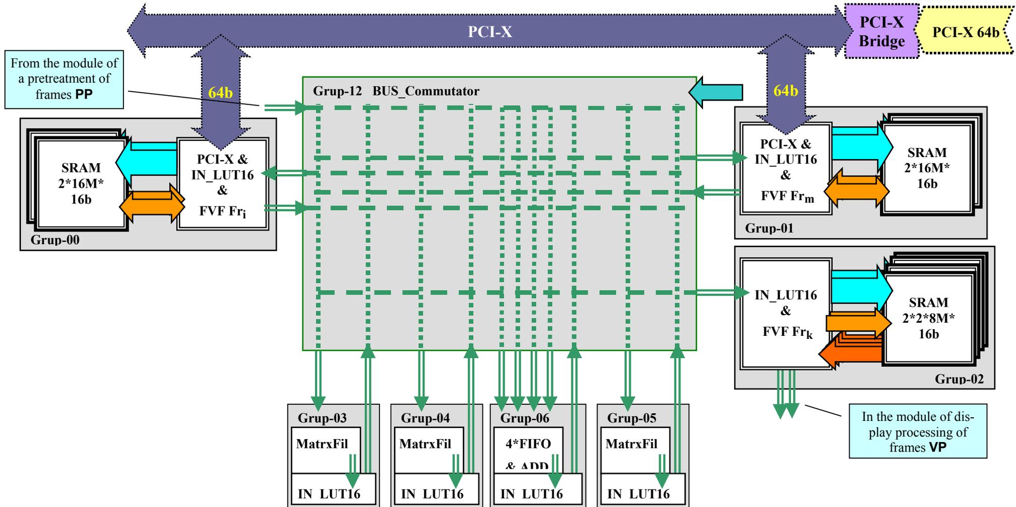
The input frame buffers FE  $FVF Fr_i$  and FE  $FVF Fr_m$  in FP module are double memory buffers, each to the full frame format. They perform processes of subtraction with complete frames hence should be loaded with full frame data and should contain all frames necessary to perform subtraction procedure as frames required differ in timing and sequence.
